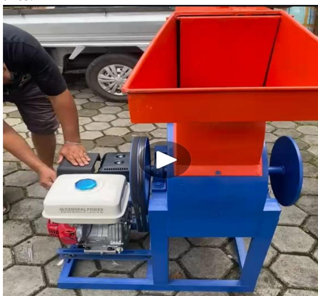
Figure 3. Plastic Shredding Machine Provided to the Waste Bank
